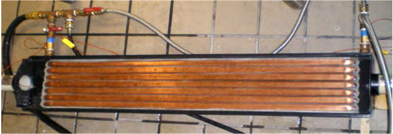
Figure 3: Ecodrain A1000 with Plastic Cover Removed
