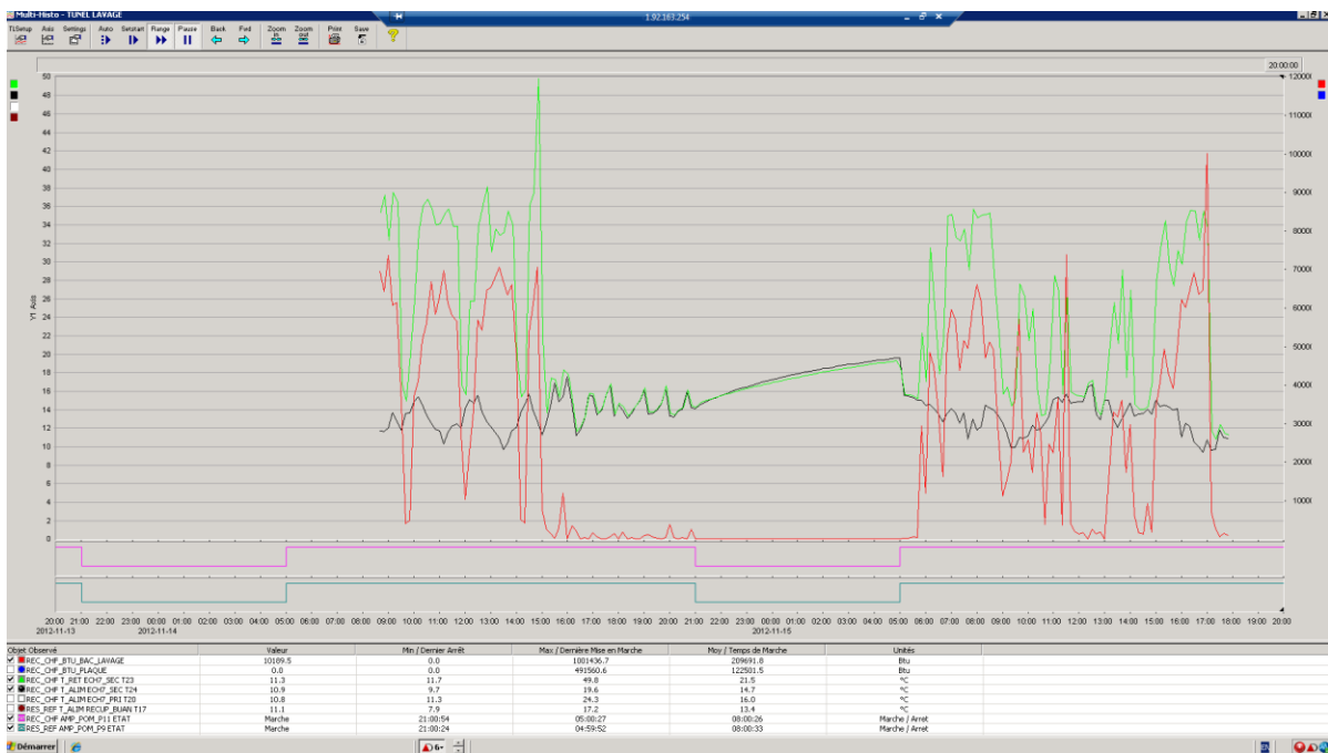
Image 3 – Real time heat trace chart indicating the substantial heat recovery (pre-heating of cold water) in the hospital laundry system, achieved by installation of the modular Ecodrain M1000 heat exchanger system.
